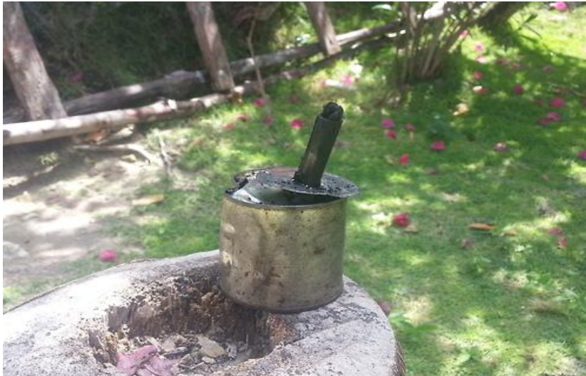
Pictured above: A Homemade Kerosene lamp called "Tet Gridap" in Ile a Vache
