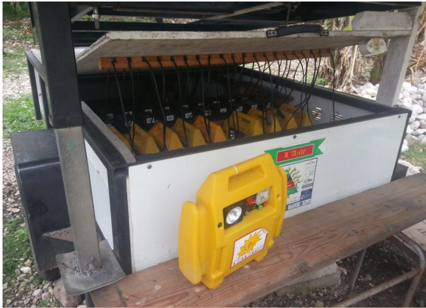
Pictured: Sirona Battery Packs "Ty Soley" and Charging Station
